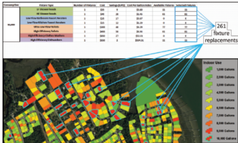
Figure 10 – Linking linear programming output back to parcels: The results of the linear programming tool can be related back to the candidate accounts or parcels in GIS.
